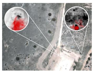
After 4 years of development, final production tests were performed in collaboration with partners in Queensland, Australia. Sensitivity tests were completed using a fixed wing aircraft over an area of controlled gas releases of varied gas volumes in a blind test.
