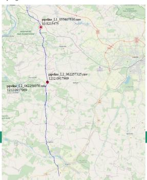
Over the course of the pipeline one controlled reference leakage was utilized to check the sensor performance and one further unknown leakage was identified and mapped shown in the picture below. While the pipeline corridor is visible from the air, the pipeline itself mainly routed through an agricultural area covered with soil and vegetation the leakages were clearly recorded.
