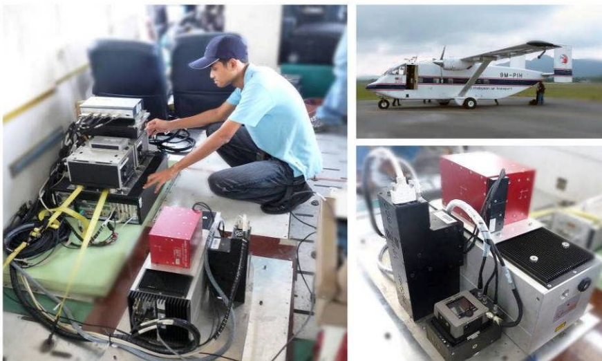
Figure 8 Airborne HySpex VNIR 1600 systems installations
